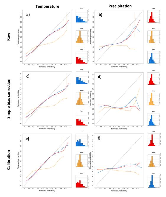
**Figure 2.** SEAS5-JRA55 reliability diagrams for Europe and JAS season (start date on the 1<sup>st</sup> of June) for 2m temperature (left column) and precipitation (right column) considering the period 1981-2015. (ab) Raw forecasts, (c-d) simple bias correction and (e-f) calibration. Red refers to the above-normal category, yellow to the normal and blue, to the above normal.
