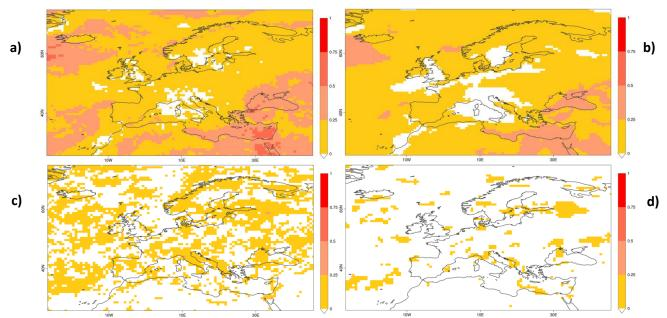
**Figure 3.** Left column: FRPSS of 2m temperature (a) and precipitation (c) obtained from SEAS5 calibrated with JRA-55 reanalysis for JAS season (start date on 1<sup>st</sup> of June) over Europe considering the period 1981-2015. Right column: Same as previous column but for FCRPSS.
